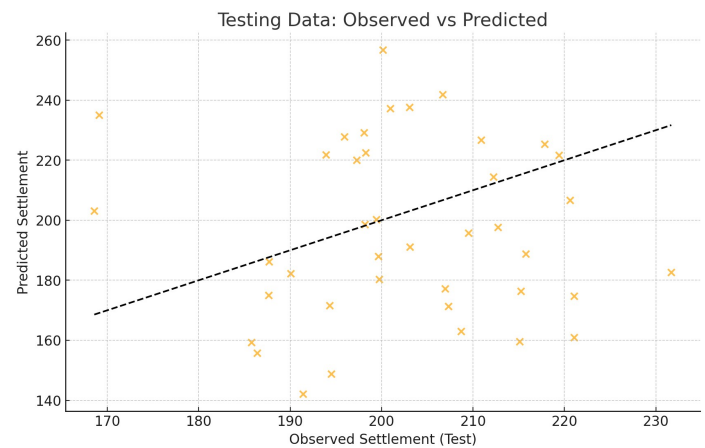
Fig. 4 Testing data for observed vs predicted settlement
